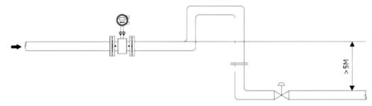
No bubbles shall be observed in the pipe.
