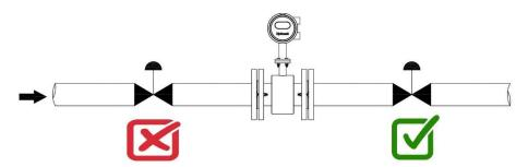
The electromagnetic flowmeter cannot be installed on the suction side of the pump.
