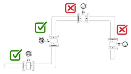
Installation of the sensor after a control valve is not recommended.
